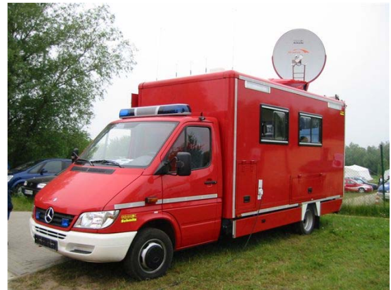
Mobile communications van with SkyRAY Light 1200 antenna subsystem
