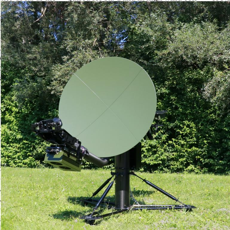
**ND SatCom's MFT-1500 is a lightweight, multi-band terminal that can withstand extreme weather conditions of up to 100 kms gale-force winds. It can be easily set-up in 30 minutes by two personnel.**
