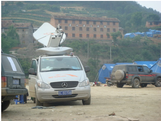
SNG vehicle with ND SatCom SkyRAY Compact antenna subsystem
