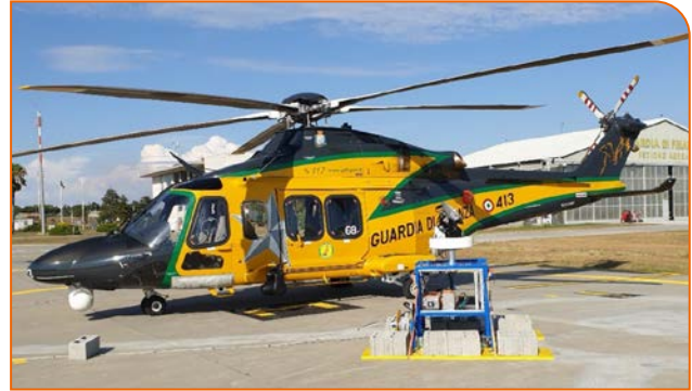
AW169 HELICOPTER IN UNDER-THE-ROTOR TESTS WITH THE HELICOPTER ANTENNA
